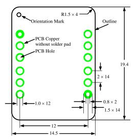
Figure 6 Top Side PCB Foot-print for the DIP Package
