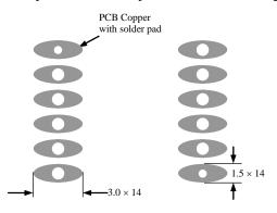
Figure 7 Top View of the Bottom Side PCB Foot-print
