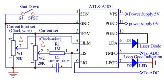
Figure 3 A Typical Stand-alone Application Schematic
