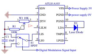
Figure 4 Low Noise Digital Modulation Circuit
